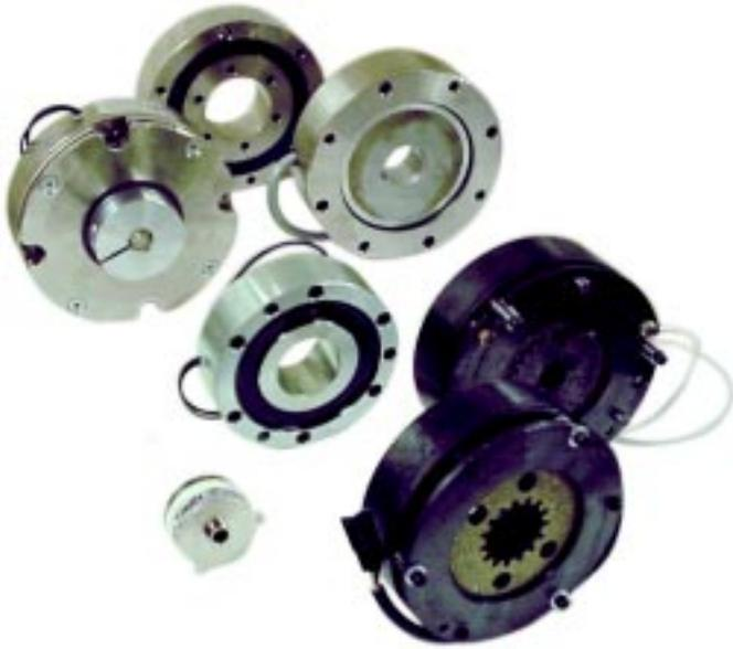
The Hilliard family of brakes are engineered for maximum flexibility and long, dependable service life. Our electric brakes are electromagnetically released when voltage is applied and spring-engaged when current is interrupted. They provide reliable routine or emergency stopping and holding.
