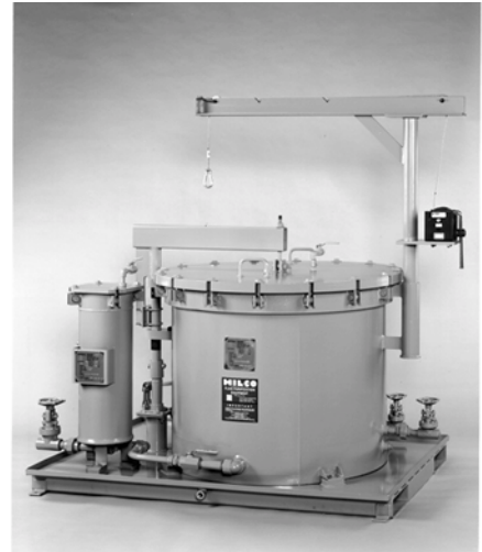
This system is designed to house six 11x19 ion exchange cartridges for a total of about six cubic feet of media. The post-filter (second stage) contains a HILCO PH718-12-CN cartridge for particulate removal.
