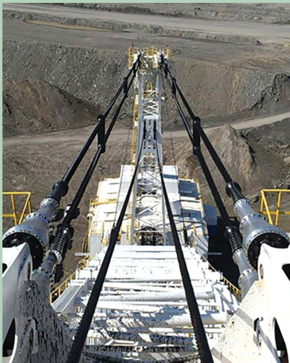
These synthetic main boom pendants provide better dampening to system movement.
