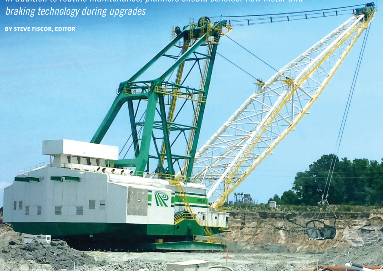
The 8200 above is one of the four draglines Flanders has converted from DC to AC power.
