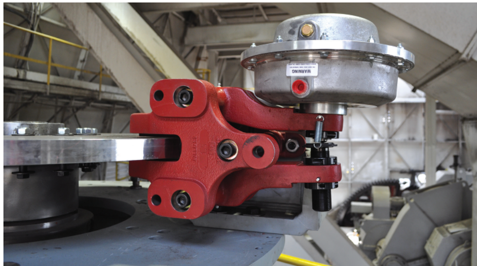
The same type of Hilliard brake, a caliper that is spring-applied and pneumatically released, can be used for all three motions.
